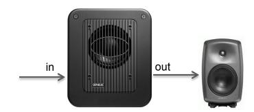
b) In parallel via a split cable to feed both the subwoofer and each appropriate monitor.
